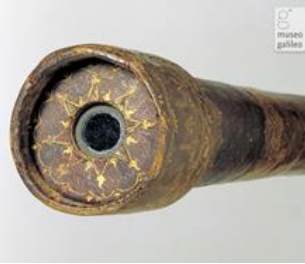
Above: The telescope used by Galileo to see the moons of Jupiter. The objective end held a plano-convex objective (now cracked), the convex side facing outward, 37mm diameter, 15mm aperture, 980mm focal length (f/65). Magnification 21X. Right: Eyepiece holders (top & bottom). Left: A 10' tall Armillary, representing Ptolemy's geocentric view of the heavens.
