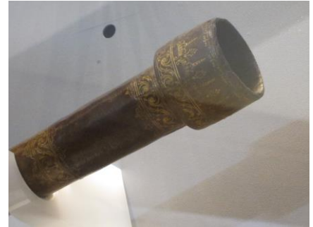
Above: The telescope used by Galileo to see the moons of Jupiter. The objective end held a plano-convex objective (now cracked), the convex side facing outward, 37mm diameter, 15mm aperture, 980mm focal length (f/65). Magnification 21X. Right: Eyepiece holders (top & bottom). Left: A 10' tall Armillary, representing Ptolemy's geocentric view of the heavens.
