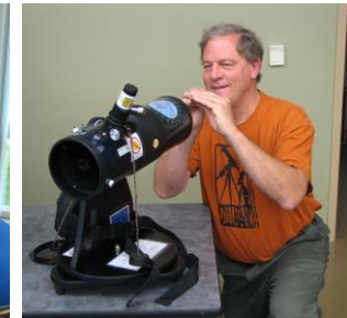
The collimation exercise involved Marc, Jeff, Bob, Rob and Rex (not shown). The modified collimation bolts behind the mirror cell, once tightened in adjustment, hold their setting for a long while, thanks to a dab of epoxy used on the nut .
