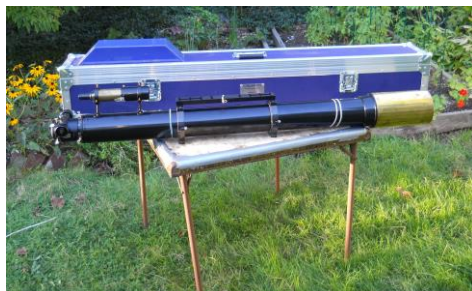
Modification to blue ScopeGuard case by Joe Derek to accommodate the semi-permanently attached finderscope and its brackets (outside and inside views). (All Photos: John Bishop)
