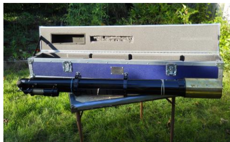
Modification to blue ScopeGuard case by Joe Derek to accommodate the semi-permanently attached finderscope and its brackets (outside and inside views). (All Photos: John Bishop)
