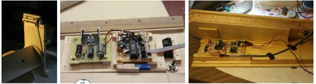
(Left): The OTA saddle and the Dec sector drive. (Center): The drive power supply and controller, with a ribbon cable that allows for firmware updating. (Right): The drive electronics are all mounted inside the north leg, with access from the top.
