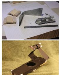
the collimation of the optical path. The slider would glide on a pair of brass rods and its lateral movement would be controlled by a threaded screw manipulated by the focuser wheel.
