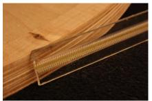
(Left): Making the worm teeth in Lexan by pressing a brass threaded rod into a strip of Lexan carefully heated up with a hot air gun. (Above): A finished Lexan worm teeth strip is ready to be attached to the Right Ascension sector.
