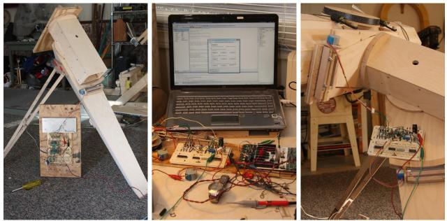
(Left): Initial test of Right Ascension sector drive with the large proto-board driver. (Center): Writing assembly language code for the controller (the watch in the foreground is to confirm the motor rotation rate). (Right): Testing the proto-board version of the final circuit on both the RA axis (lower right) and the Dec axis (upper left). The blue 'knobs' are the two step motors.
