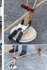
(Left): Ian pressing down on the mount as part of the "Ice Test" of the single strut. (Center): A south leg with a wood and Teflon pad underneath to promote slippage (above) and a
