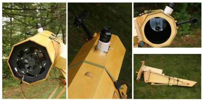
The cooling fan for the mirror cell (left), the barrel focuser on the sled, whose lateral movement is controlled by the focuser wheel visible in the middle (center), the look down the OTA at the mirror (top right) and the compact folded disposition of the Mount (right), that being a prime objective. Beauty as seen through the optics, both celestial and terrestrial (below). Clockwise from the left: The Dumbbell nebula (M27), the eastern end of the Veil nebula and a daylily in the garden.
