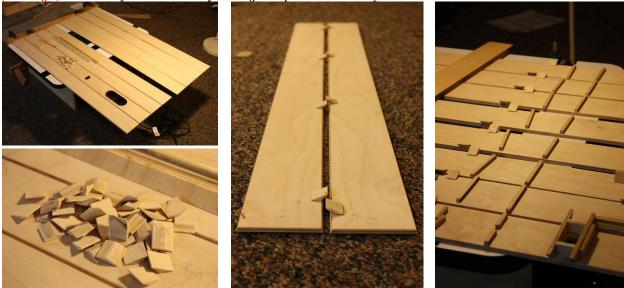
Parts of the OTA laid out for assembly. The eight sides of the tube (top left) and some of the custom fasteners (bottom left, center and right above) come together to make the tube for the 6" mirror. The tube was glued into two halves (far left below). The groves and rods the sled focuser slides on (center and right below), with its lateral movement controlled by the focuser wheel rotated from outside the OTA.
