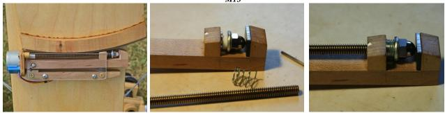
(Left): The Stellafane version had the acorn nut, but not the sheet of aluminum. (Center and Right): The post-Stellafane version shows the plastic bushing used to control the spring that keeps the acorn nut pressed against the aluminum surface.
