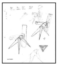
The "Hawaii" telescope was built to fit in a suitcase and was taken to Hawaii for the 1991 Total eclipse. A driven equatorial fork mount designed to carry a lightweight 500mm f/8 lens (costing \$69) with the option of a 3" f/5 achromatic refractor, the scope was featured in *Sky & Telescope's Gleanings for ATMs* (May 1992).
