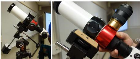
The Lunt on the EQ1 mount (left), with the special mods for secure fastening (right).
