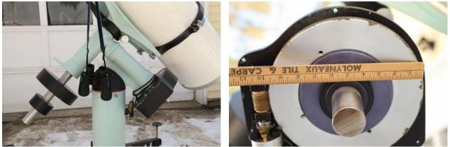
Close-ups of some of the finer points: the EQ head (top left), the clock drive gears (top right) and the Declination fineadjustment arm (below left), as well as the removable wooden platform with a 60mm finder and a Telrad (below right).
