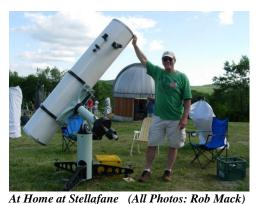
All the bolts and fittings are either stainless, brass or aluminum. The counterweights are 10lbs and 75lbs. A 12-inch tangent arm with threaded brass rod provides a smooth declination fine-adjustment. A similar hand-adjustment is located on the pier for changing the polar shaft's altitude. Stainless/brass leg-levelers stabilize and level the mount after it has been rolled out on small casters.
